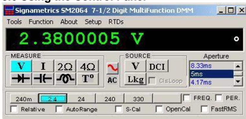
Figure 3-2. The Control Panel for the SM2064. The three main groups include Measure, Source and Range buttons. The Range buttons are context sensitive such that only “240m, 2.4, 24, 240 and 330 appear when in AC Voltage Function is selected, and 2.4m, 24m, 240m and 2.4 appear when AC Current functions is selected, etc.
